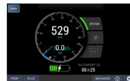
Propulsion: regeneration mode
